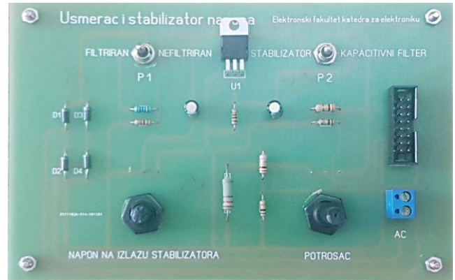
Fig.1 - The breadboard with full-wave rectifier (left) and voltage regulator (integrated circuit in the upper middle position of the board). The measuring unit is connected via IDC connector, positioned at the right side of the board.
